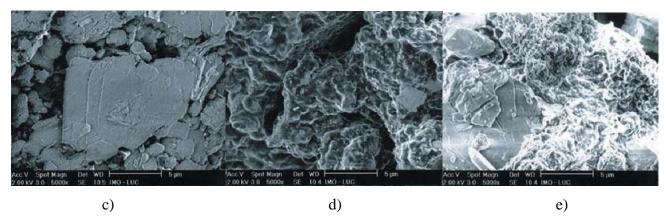
**Figure 3** SEM pictures of GTR produced in different ways:ambient (mechanically ground)
