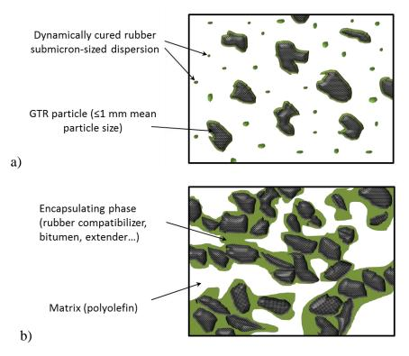
Figure 5 Morphology of thermoplastic/GTR blends: dispersed (a) and co-continuous (b)
