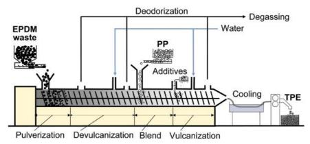
**Figure 4** Dynamic devulcanization and dynamic vulcanization processes for the product of TPE based on EPDM waste [45] (Reproduced with permission)
